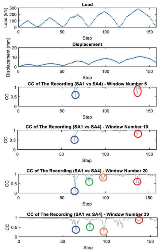
Figure 5. Comparison amongst load, displacement (maximum deflection) and *CC* of SA1-SA4 sensor pair over load steps. The circles represents the formation of a major crack (see Figure 7 for the color code).
