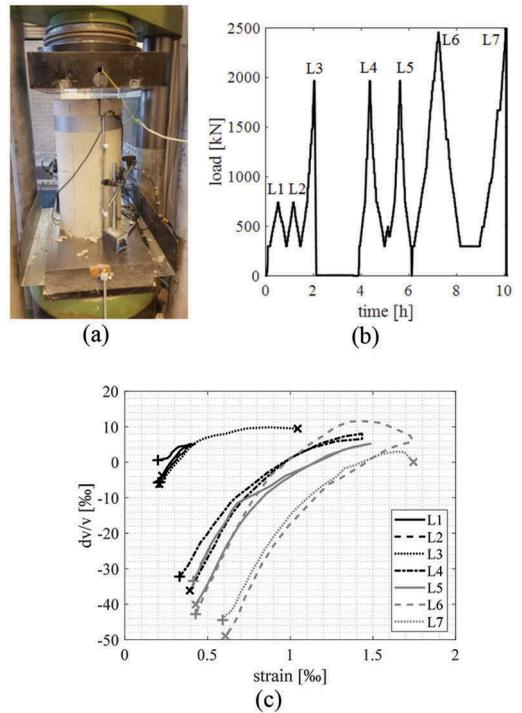
Figure 1. (a) Cylinder specimen test setup, (b) loading history, (c) wavespeed change with strain.
