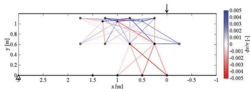
Figure 4. Wavespeed change at load level 150 kN compared to the unloaded condition.
