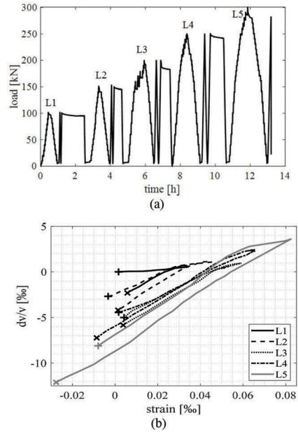
Figure 3. Beam-specimen tests: (a) Loading history, (b) wavespeed change vs strain.
