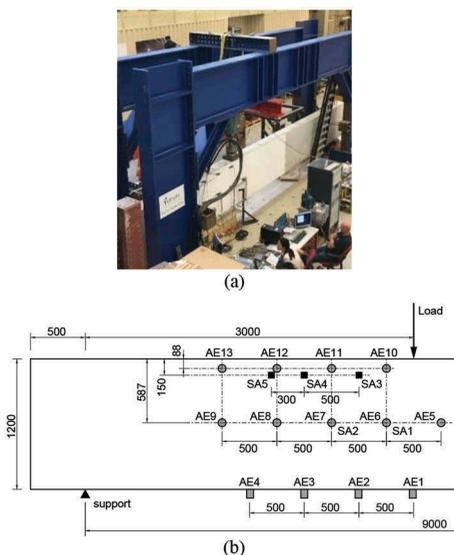
Figure 2. Beam specimen: (a) Test setup, (b) Sensor layout.
