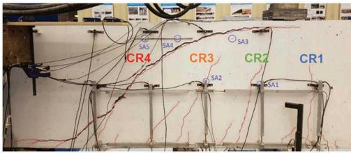
Figure 7. Locations of SA with respect to the final crack pattern.
